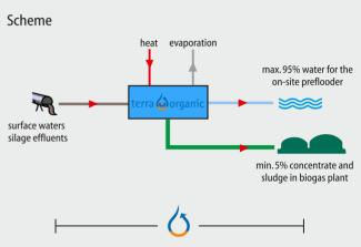
The volume that can be treated per TerraOrganic module depends on the selected concentration level. This is determined by the admissible water volume in the fermenter and may be fixed individually by the operator.
